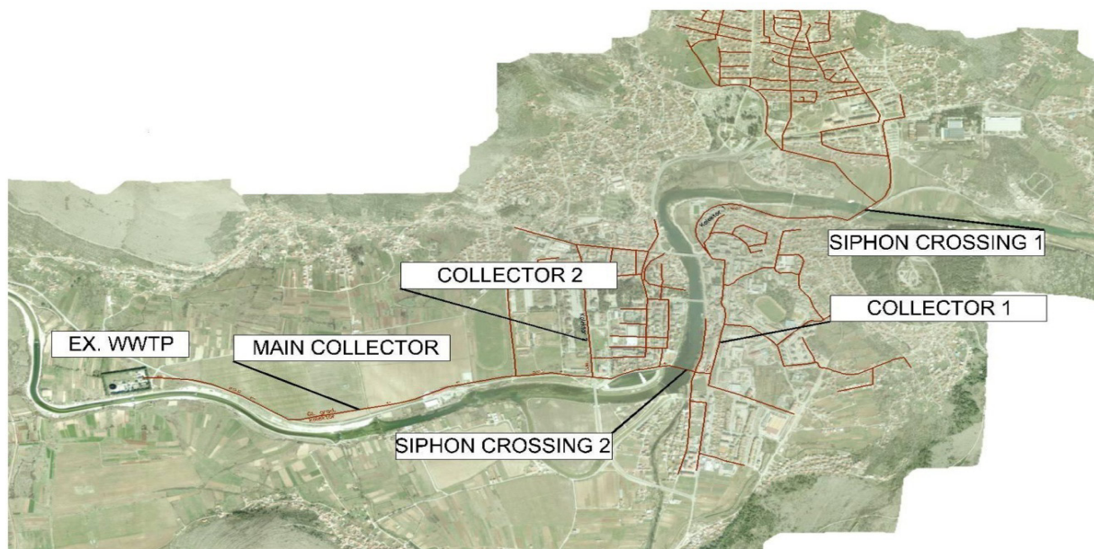
Figure 4-44 – Layout of key components of existing sewage collection and treatment system
